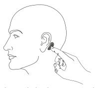
6. Then simply snap the hearing system onto the adhesive adapter using the coupling.
